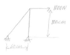
4. For the beam shown in figure. Compute slope at the hinged support points Modulus of Elasticity E=200GPa and  $I=4\times10^6$  m<sup>4</sup>. Use two beam element.
