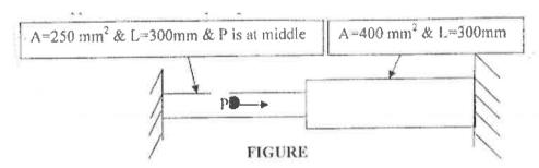
3. The members (1) and (2) are circular in cross section with diameters of 10cm and 20cm respectively. Determine the displacement at the node where load is acting as shown in figure. Take  $E=2\times10^6$  N/cm<sup>2</sup>.
